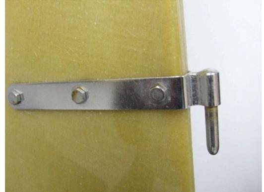
Another part that may need replacing is the bottom 3-hole rudder pintle. Check the corners up near the pin. Frequently the weld will break or the corner bend will tear. Evidence of this failure is visually evident long before the part gives way.
