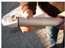
Apply a heavy coating of silicone sealant to mast extender in an effort to make a watertight seal with mast and to keep it attached. Slide together and wipe off excess silicone.
